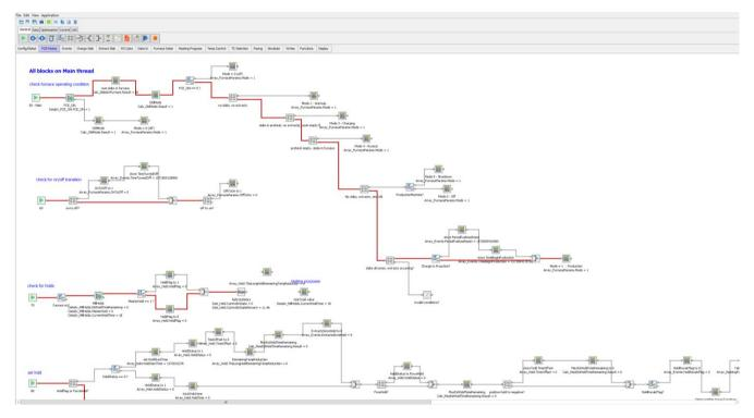
Example of application logic from the Griffin graphical programming environment. Logic can be added, removed, or transformed in any way and redeployed without interruption of control. While applications are running, the execution path is highlighted in red.
